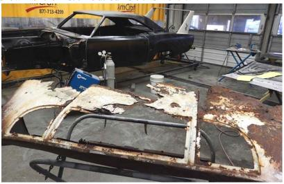
Both cars from the woods were pretty rough. The white car had a tree growing into the corner of the nose. The bottom of the nose was very bad with rust, and corrosion had taken a toll on the floor pans and roof of the body. The front and rear rail areas were good. And it is a numbers matching car with build sheet and one hundred percent complete as well.
