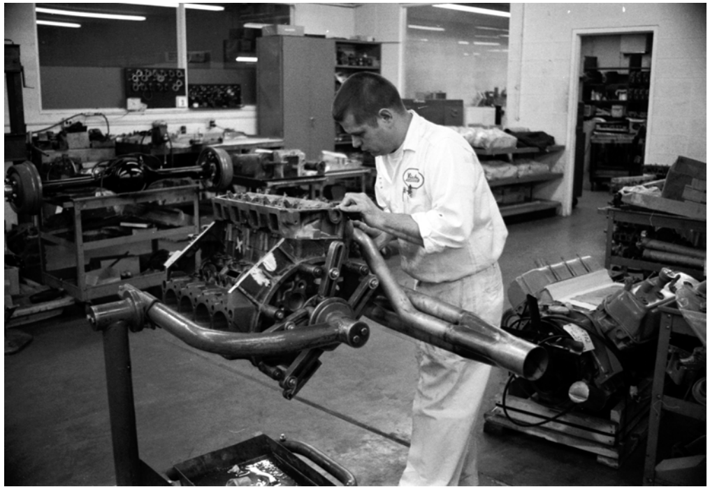
Minnie Joyce works on a race Hemi in the shop at Nichols Engineering, circa 1969-70. Note the beautiful stainless header. Engine NH-902 (Nichels Hemi #902) sits on the floor in the background. Every Nichols built engine was documented like this.
