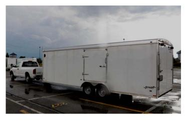
One of the problems with the old 1997 built trailer is that it had torsion axles rated at 3500lbs each. The trailer probably weighs 3000 lbs. Put a 4000 lb car in it, plus a little crew gear in front of the trailer and you guessed it, we are overweight. It has been explained to me that the entry level box trailers with the light duty axles are made for the low price point and for landscapers or people not hauling a heavy car.
