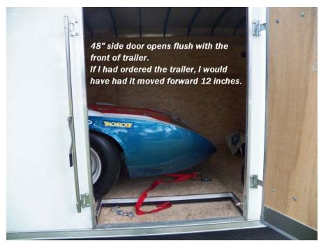
The normal entry door on the passenger side is 48" Because of the position relative to the nose on the Superbird, I would also consider moving that door forward twelve inches. My nose cone covers about half of the door opening as positioned. My old trailer had a 36" door and was it was thus in a better position.
