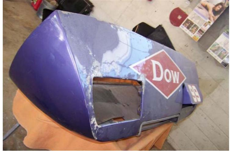
Wayne's Cyclone Spoiler II is a Cale Yarborough Special. The body is in pretty good condition and it's currently stripped for repaint. Below you can see the details of how a Talladega or Spoiler II fender is put together with both a vertical seam where the cap is attached and a horizontal seam near the top edge of the fender.
