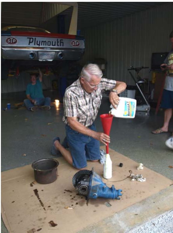
Above: Ramo is loading up some Unocal grease for the rear end. The steel can next to the rear gear is a special storage case the teams used back in the old days.
