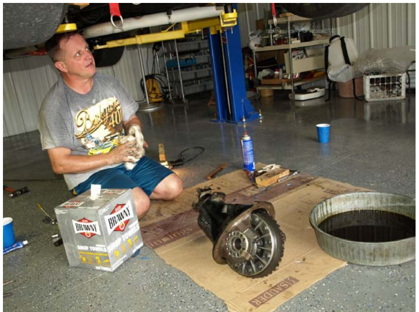
Above, Corrie has the new gear ready to go back in. The old ratio was a 3.23 which with the size of tires, feels more like a 2.50. The new set is a 4.75 ratio which Ramo says he used on mile dirt tracks in other cars. Below: Ramo is all smiles letting the car down off the lift. With the exhaust dumps on, it takes some work to get the lift pads around them.
