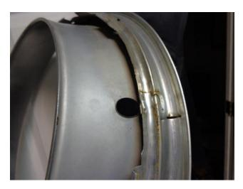
Left: Incorrect aftermarket trim ring with large GM oval valve stem hole. Retainer is different and may not have the styling ridge on the face. Right: Correct 15 x 7 Mopar ring.
