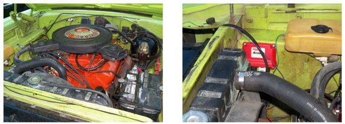
With the air cleaner on, it is difficult to tell there is no carburetor on the car. The power module is mounted on the right hand fender apron. It could be mounted out of sight if desired. The power module controls all high current functions. It connects to the throttle body ECU, oxygen sensor, fuel pump and controls fan functions. The entire system consists of only eight wire connections.
