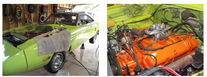
Less than a week before leaving for Colorado and the car is nearing fire-up. It is also getting a complete Accurate LTD exhaust system which overall, fit up very nicely. The oxygen sensor bung provided with the system was added to the new H-pipe. On the right photo, the factory stock linkage from the old carburetor was used. The only adaptor bracket needed was a U-shaped bracket Chuck had on the shelf when he ran a Holley carburetor.
