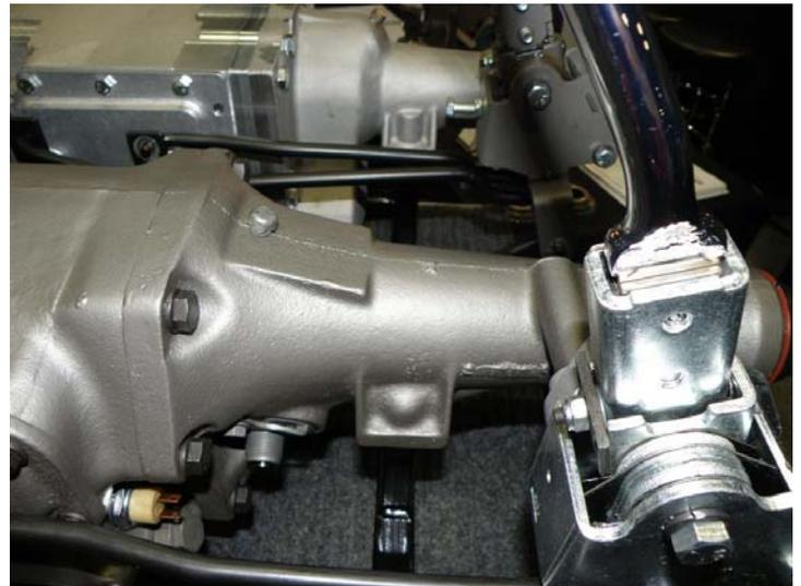
These little details just should put this product head and shoulders above any other option out there as being a true bolt in with no mods. Jamie says there should be no doubt as to the direct fit and finish of this product. The photos above are the factory A-833 4speed (four bolt flange) and the Passon 5-speed with the five bolt flange.
