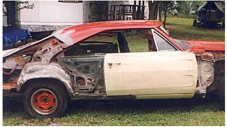
Above left is the donor unibody side getting ready to go on the car. At right, it's welded on and the door fitted. This was an ambitious project, for sure.
