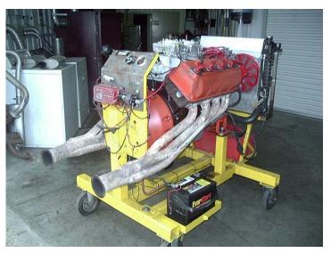
Outside was an engine test stand with a customer's fresh Hemi they fired up for testing. Open headers of course! Everyone loved the noise, not to mention it's a great service to be able to provide. Over on the assembly area sat a Challenger T/A being tweaked. You name it, from body and paint, mechanical, wheel alignment, machining, these guys can do it all.
